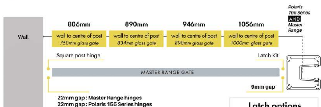
Master range square post hinge set Set of 2 MR-SPH-P/S/B
